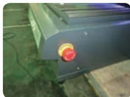
Emergency stop device system
